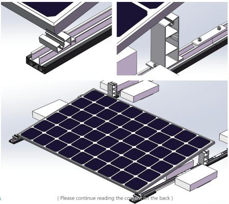
4.2 Bottom clamp installation: press the bottom clamp into the card slot as the picture shows, lock the bolt, and press the panel tightly
