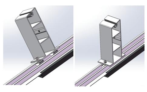
2.3 Repeat the above steps to install all front and rear legs, making sure that the top surface of the front/rear legs in the same row are at the same height to ensure the normal installation of panels
