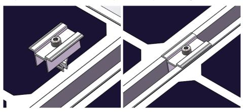
4.5 The remaining end clamp installation: place the panels in sequence according to the drawing as the picture shows, on the other side of the same row of panels, repeat steps 4.2/4.3
