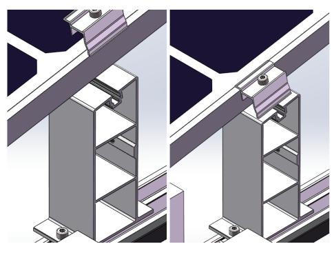
4.4 Inter clamp installation: place the panels in sequence according to the drawing as the picture shows, and place an inter clamp between two panels, then tighten the bolts
