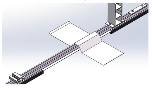
3.2 Place the ballast on the ballast plate
